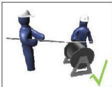
Correct method for laying the rope
