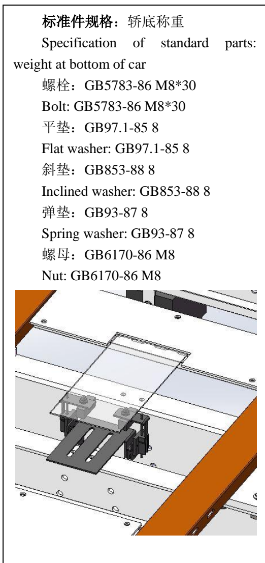
图 13-3 轿底称重安装示意图 Figure 13-3 Installation Diagram of the Weigh of the Car Bottom
