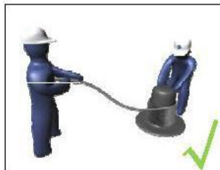
Correct method for laying the rope
